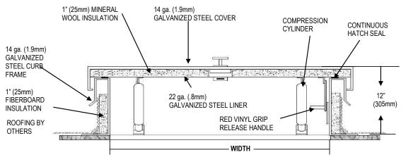
Curb: 14 ga. galvanized steel. 12" high curb with 3-5/8" wide flange including holes for securing to roof deck. (Curb includes integral counter flashing)
