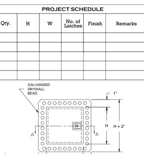
WALL OPENING = DOOR SIZE + 3/8" INTERIOR W 1 LATCH SPRING RELEASE W + 2" CLIP SPRING 2 5/8' EXPOSED 16 GAGE DOOR HINGE 5/8" FIRE CODE GYPSUM BOARD KEYED CYLINDER AROUND ROUGH OPENING PADDLE LATCH SECTION A-A Made with Union Labor
