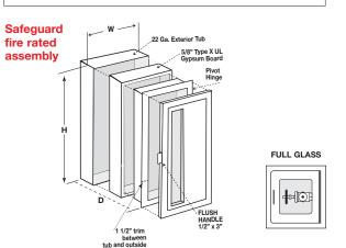
SAFEGUARD Sonoma Series VC-SN Valve Cabinet Knockout Drilling: No knockouts are provided with Sonoma Safeguard Valve Cabinets. Find the exact location of the pipe(s) which enter the cabinet and mark the cabinet tub appropriately. Both outside and inside tubs and insulation material must be completely open to receive pipe(s).
