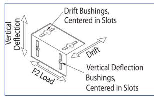
Fastener Pattern 1 replicates a condition of out-of-plane wind or seismic force with no vertical live load deflection or in-plane drift.
