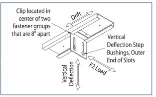
Fastener Pattern 1 replicates a condition of out-of-plane wind or
