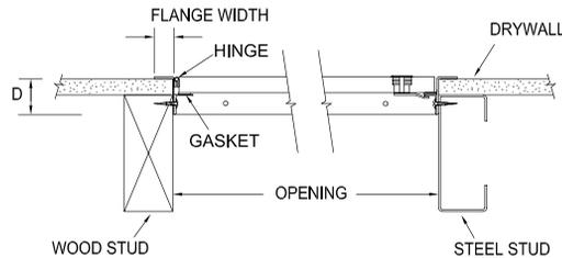
Model NGP met the performance criteria as per CSA A440-00 (windows) for an Air Infiltration of A-3 for both 75 Pa and 300 Pa, for Air Exfiltration the sample met an A-3 rating at 75 Pa and A-2 rating at 300 Pa. In Water Tightness by Static Pressure the door sample met a B-1 rating, subject to using an optional watertight mechanism, phone for details. Testing performed by Intertek (Warnock Hersey).
