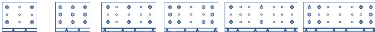
4 Screws, Pattern 1 9 Screws, Pattern 2 6 Screws, Pattern 3 10 Screws, Pattern 4 6 Screws, Pattern 5 10 Screws, Pattern 6
