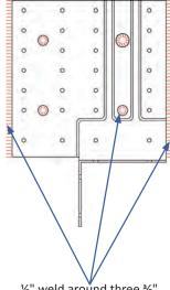
½" weld around three ¾" diameter holes, one ½" diameter hole, with ½" welds along each side.
